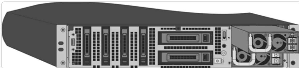
Figure 4. Insert the Replacement DC Power Supply
