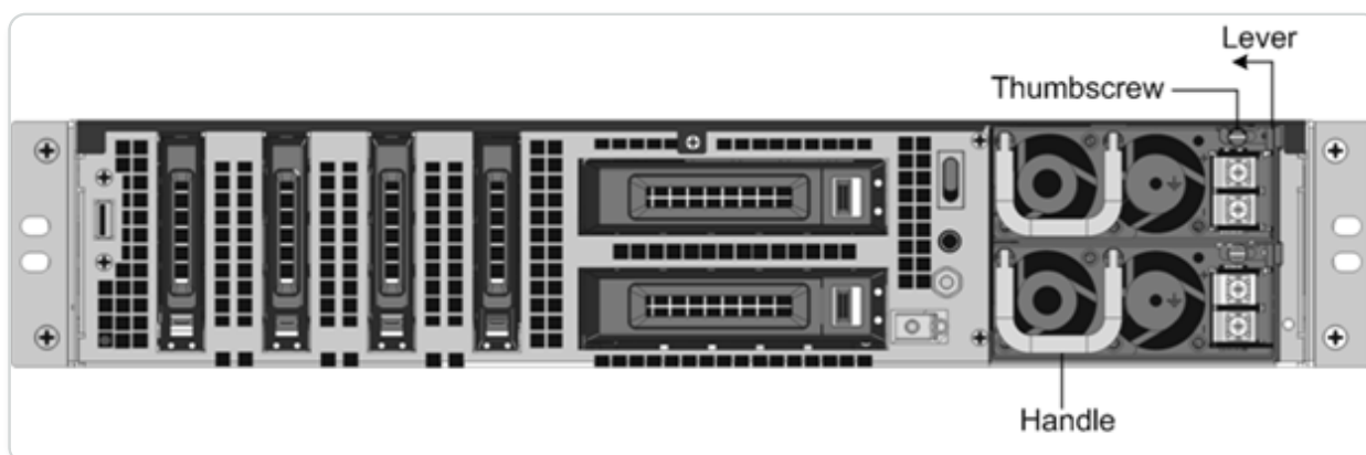
Figure 2. Remove an Existing DC Power Supply
