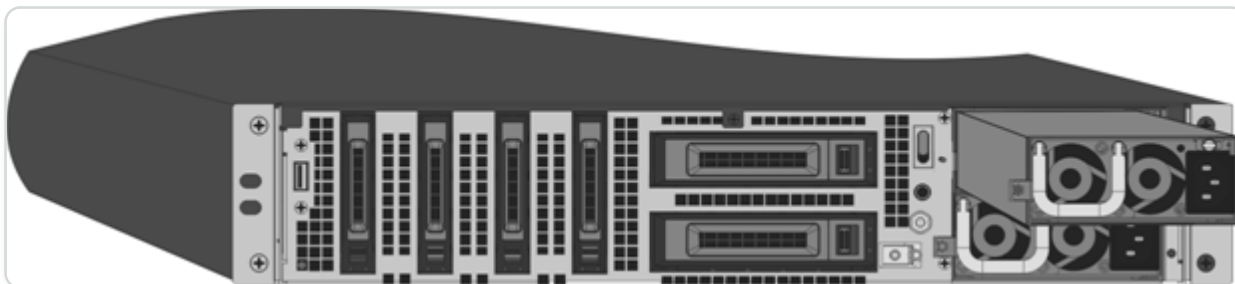
Figure 4. Insert the Replacement DC Power Supply
